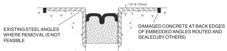
Fig. 3: BEJS SYSTEM in New or Rebuilt Joint Edges with EMSEAL Nosing Material
