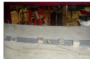
Thermocouples register no more than 248 °F (120 °C)
