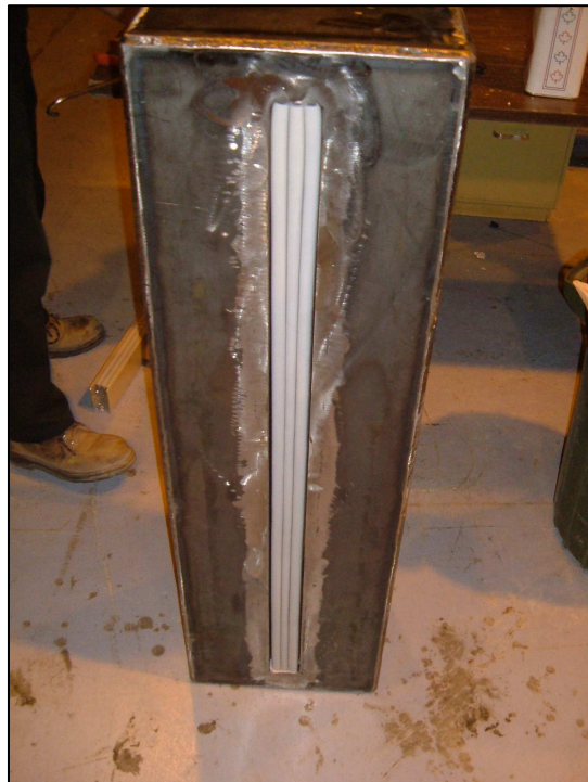
Figure A4 – Installation of Exova Specimen No.: 09-06-M0379 in Fixture
