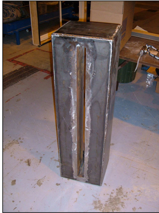
Figure A1 – Test Fixture Prior to Installation of Expansion Joint
